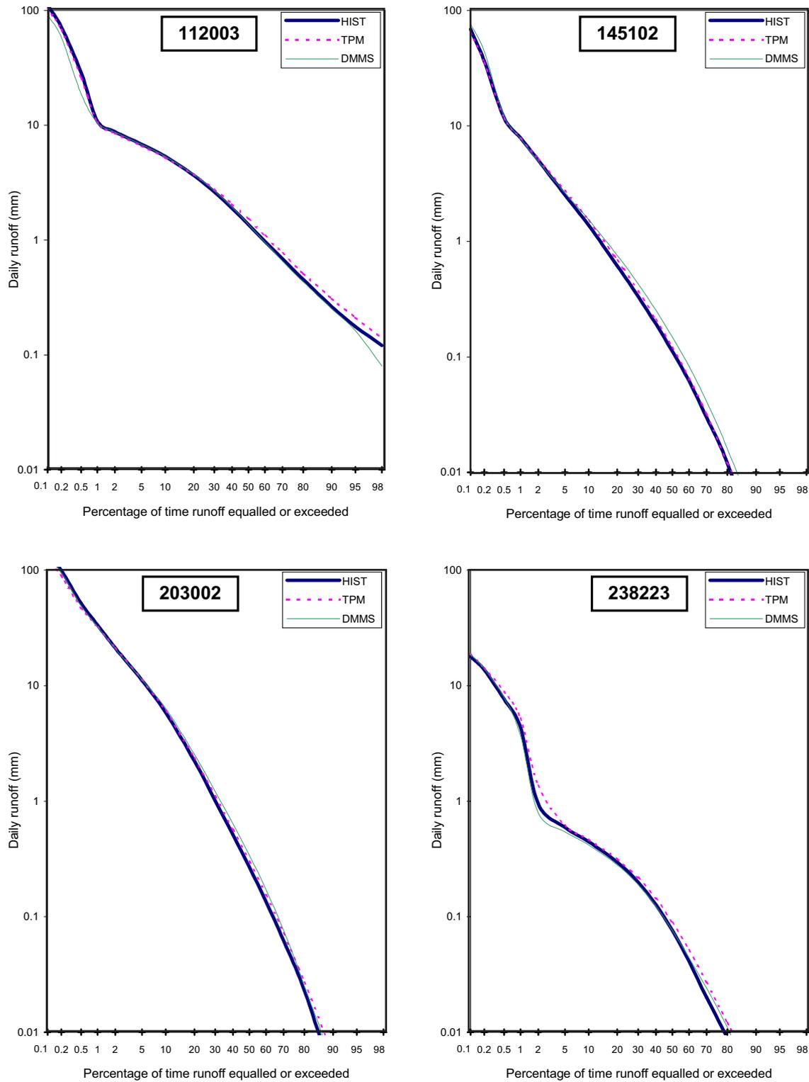
Figure C.6 Comparison of flow duration curves derived by modelling generated rainfall and historical rainfall
