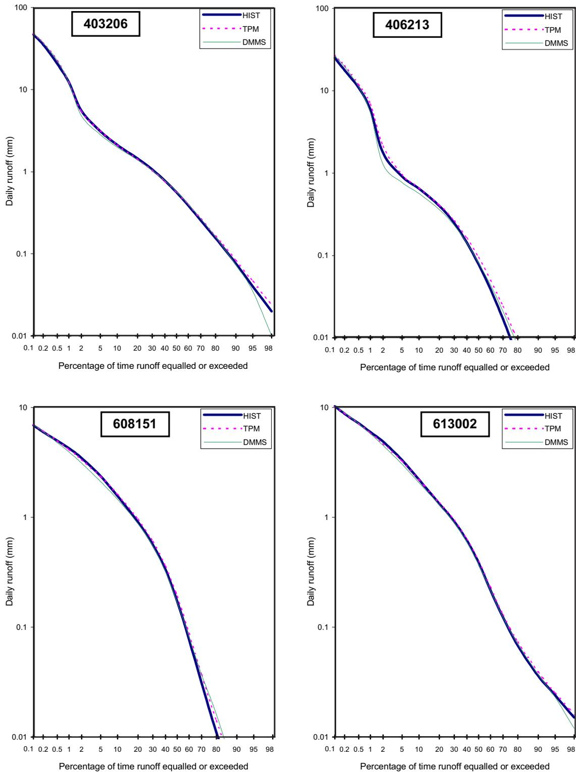
Figure C.6 Comparison of flow duration curves derived by modelling generated rainfall and historical rainfall (continued)
