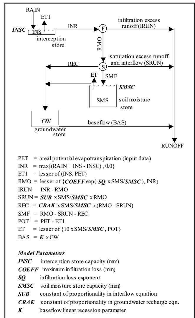
Figure 4.1 Structure of the conceptual rainfall-runoff model SIMHYD
