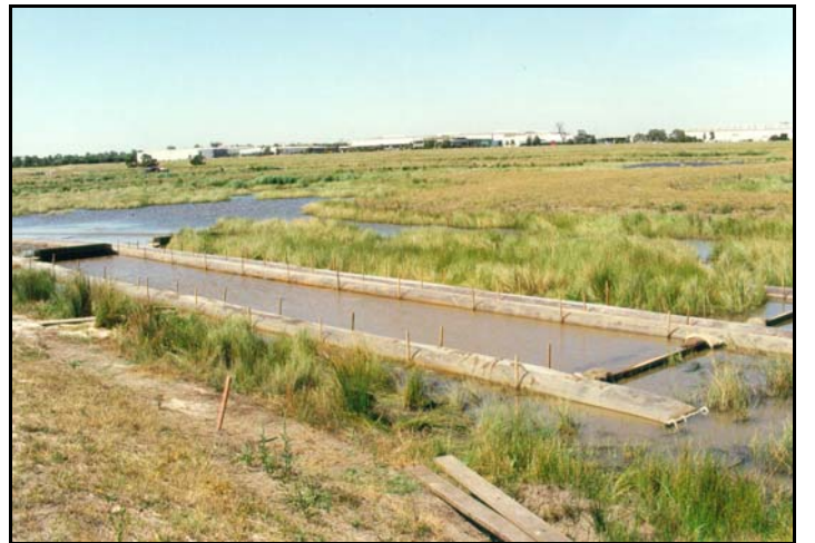
Figure 8 Experimental channels established for investigation of the role of wetland macrophytes in suspended solids removal and scalability of wetland systems.
