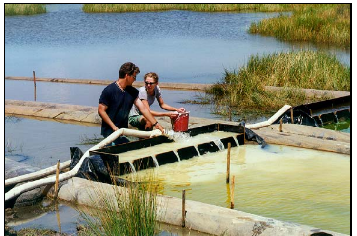
Figure 9 Dosing of experimental channels with pre-determined particle size tracer
