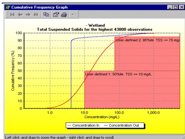
**Figure 3:** Cumulative probability plot output, showing water quality standards (shaded boxes).
